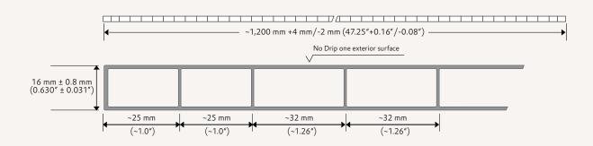
ACRYLITE® Heatstop high impact acrylic sheet is an IR-(infrared) reflecting, heat-insulating and highly weather resistant double-skin sheet made of high impact acrylic (polymethyl methacrylate, PMMA). The Heatstop component is uniformly distributed throughout the entire sheet.
