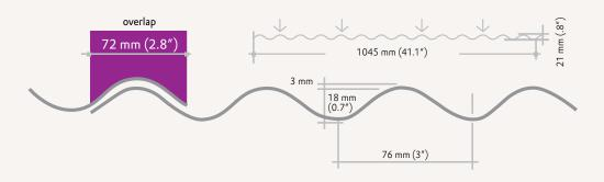
3 mm ACRYLITE® Resist high impact acrylic wave profile is a highly light-transmitting and weather-resistant sheet made of impact-modified Acrylic (polymethyl methacrylate, PMMA) polymer.
