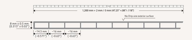
8 mm ACRYLITE\* Heatstop high impact acrylic doubleskin sheet is an IR-(infrared) reflecting, heat-insulating and highly weather-resistant sheet made of impact-modified acrylic (polymethyl methacrylate, PMMA) polymer. The Heatstop component is uniformly distributed throughout the entire sheet.
